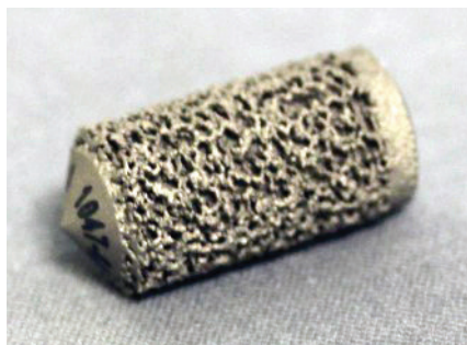
Figure 1: Bone plug with Tesera Trabecular Technology porous structure
